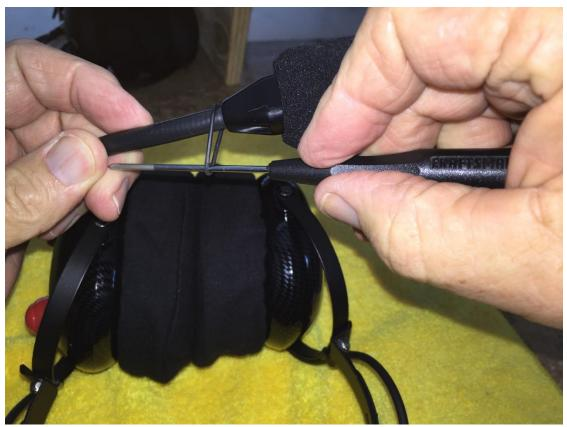
Carefully, while pulling the O-Ring out, wind it on to the Mic Boom. Don't try to pull it off over the Mic.
