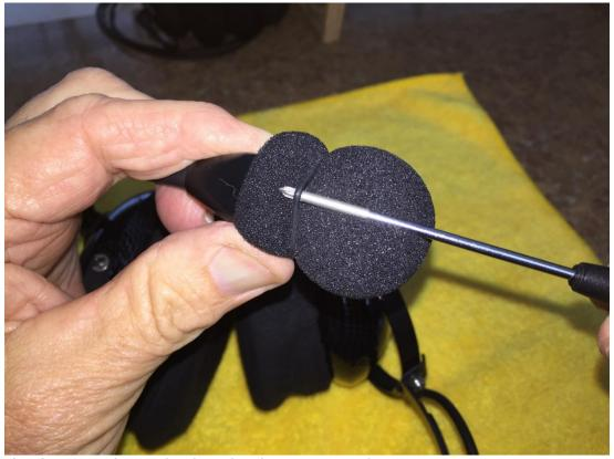
Slip the Screwdriver shank under the O-Ring Sock Retainer
