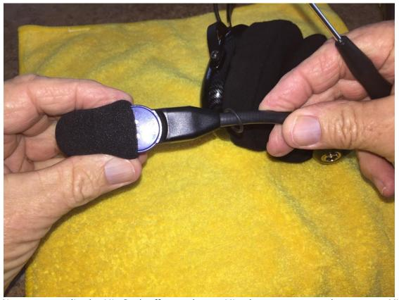
Now you can slip the Mic Sock off to exchange Mic elements or to replace a worn Mic Sock.
