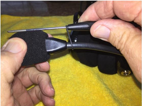
As before slide the shank of the #00 Philips screwdriver under the Mic sock and up to the Handle.
