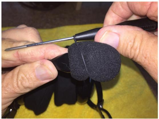
Slide the Screwdriver up to the handle as shown and lift the O-Ring away from the Mic Sock
