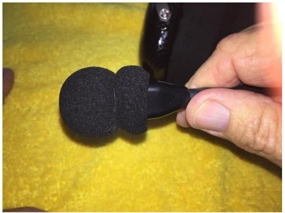
Fully installed it should look like this. If you need to even it out you may do so by grasping a large portion of the corner and pulling out over the sharp corner of the Mic holder to get it aligned. If you don't grasp enough of the Foam Mic Sock doing this final step you can pull a tiny piece off, so use care.
