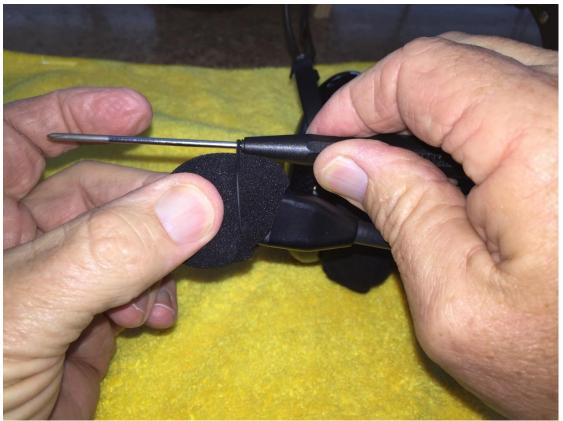
Just keep **winding** the O-Ring over the Mic Sock until it is in position at the base of the Mic Element.
